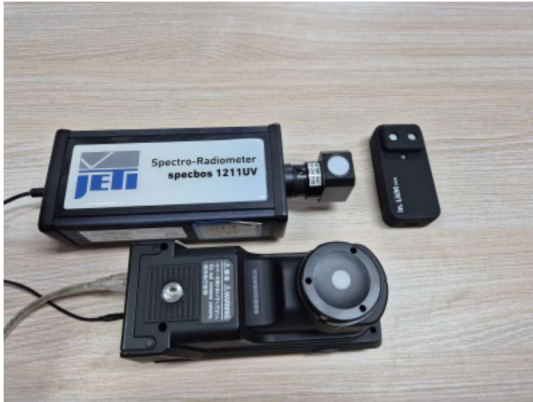
Figure 1 The three instruments used in our test: Jeti Specbos (top left), Ultra (top right) and Konica Minolta CL500A (bottom).
