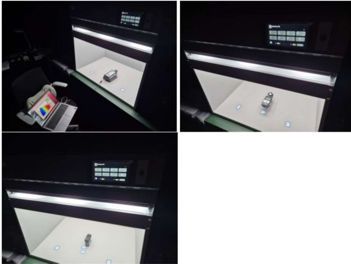
Figure 2 The three instruments, sequentially placed in exactly the same position and height inside the Thouslite GT light booth.
